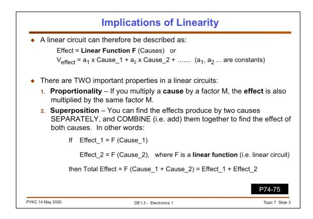
So, linearity is characterised by a linear function which is a weighted sum of variables (causes) where the weights are constants.
