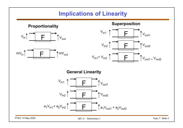
This is best shown diagrammatically. Although what is shown here are input and output voltages to a system, the same holds true for any node voltages or currents inside a circuit, and for any fixed or dependent sources (provided that the defining equation of the dependent sources also has a linear relationship).
