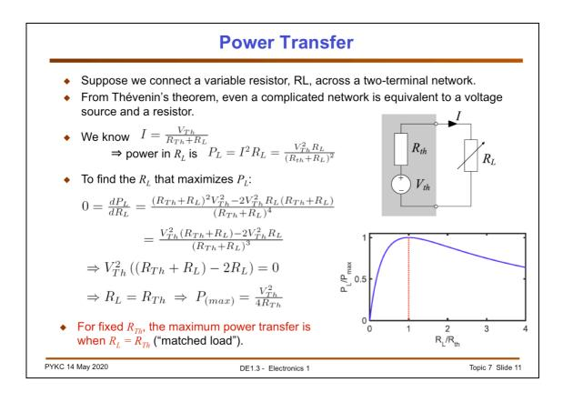
Let us consider a source with some internal resistance modelled by the Thévenin equivalent circuit as shown here. What is value is the resistor load such that the power transferred from the source to the load resistor is MAXIMUM?
