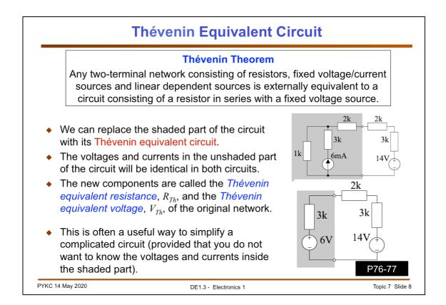
**Thévenin Theorem** states: consider a two terminal circuit (network) with only resistors, fixed sources and linear dependent sources. No matter how complex this circuit is, you can always replace it with a simple fixed voltage source in series with a resistor. So the upper shaded circuit can be replaced with the lower shaded circuit.
