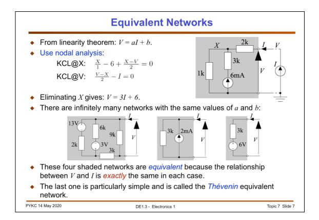
Let us consider the circuit shown here. Imagine that circuit in gray is a "**black box**", and we are interested in the relationship between the voltage V at the output of the black box, and the current I flowing into the black box. We can model this situation with the unknown current source I at the output of the black box.
