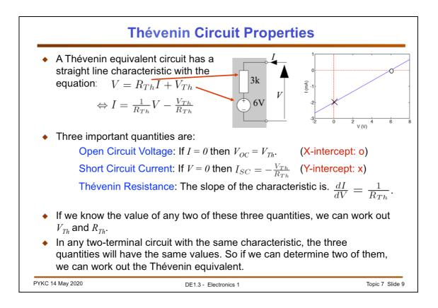
Thévenin equivalent circuit always have a straight line characteristic. (Characteristic of a component or an electronic widget is the plot between I-V or V-I, or some other electrical parameters). In a Thévenin equivalent circuit,
