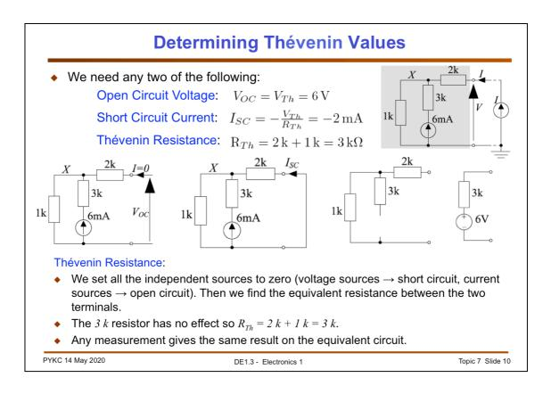
Let us consider how to go from the complicated circuit on the upper right to the simple Thévenin equivalent circuit on the lower right. Remember,
