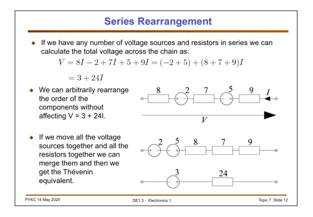
Here are some examples of how to re—arrange sources and resistances to simply circuits.
