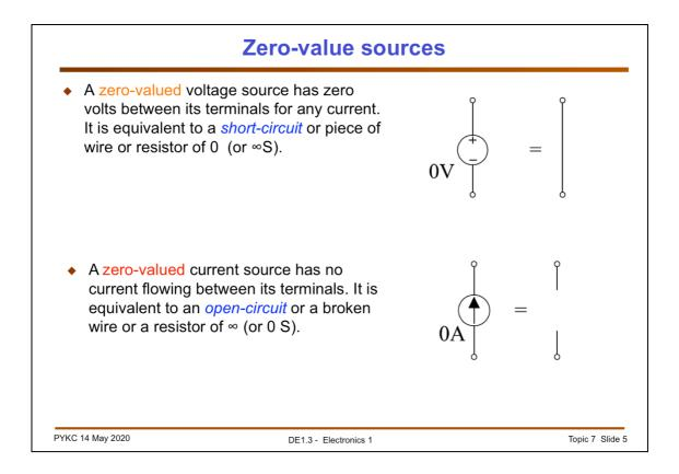
Let me further introduce the idea of zero-value sources. A voltage source could have a zero value. In which case, it is equivalent to a short circuit or a wire. If you have a voltage source with a fixed value  $V_S$ , and if you wish to "eliminate" its impact (cause) on a circuit, you can regard that  $V_S=0$ , or replacing the voltage source with a wire.
