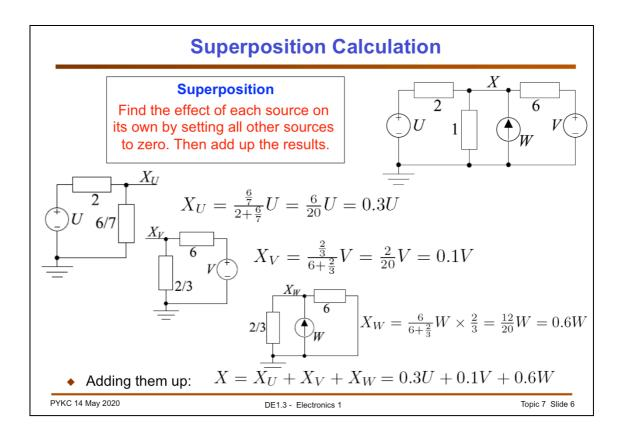
Let us apply the principle of superposition to evaluation X in the circuit shown here.
